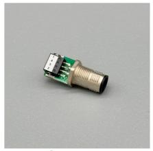
The CON-M12-4PIN-Single-AdapterMale is an adapter. This adapter was specially designed for applications where open cable ends must be adapted quickly and easily to a standard plug and a small form factor is also required. If the connection point is properly housed, higher protection levels are possible. The great advantage of the design is that the spring-loaded terminals make assembly easy and can be done under field conditions.
