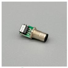
The CON-M12-4PIN-Double-AdapterMale is an adapter. This adapter was specially designed for applications where open cable ends must be adapted quickly and easily to a standard plug and a small form factor is also required. If the connection point is properly housed, higher protection levels are possible. The great advantage of the design is that the spring-loaded terminals make assembly easy and can be done under field conditions.
